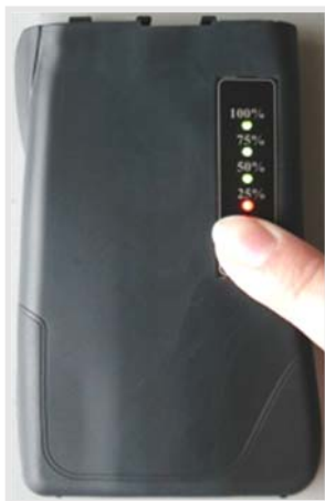
Test of battery charging condition
